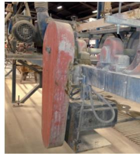
**Coveyor motor** *for waterfall application of glazes and engobes*
