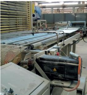
**Furnace feed conveyor motor**
