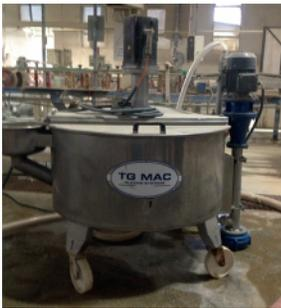
**Glaze and engobe tank motor**
