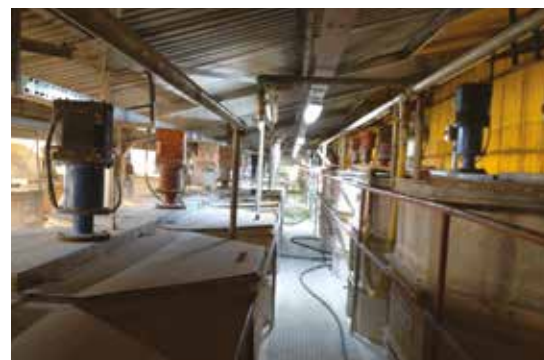
Glasur Mixer - 185 Nm - 30 rpm
